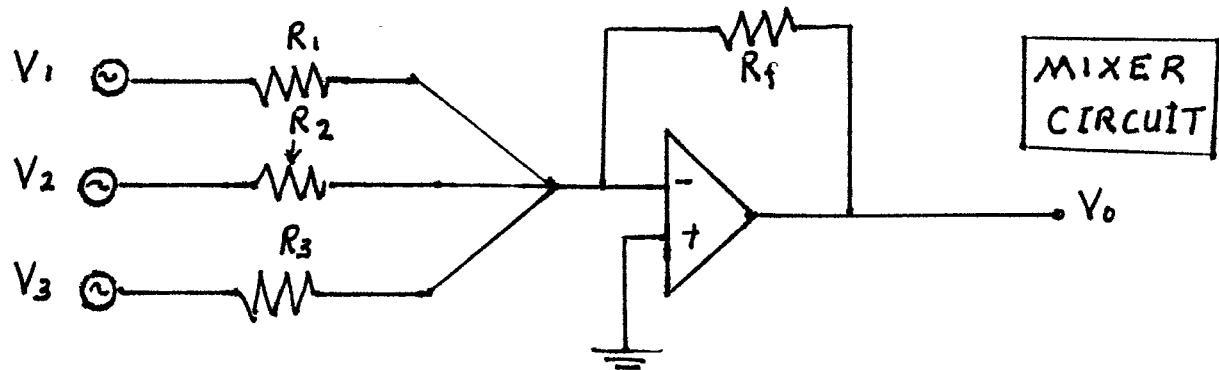
$$\frac{V_1}{R_1} + \frac{V_2}{R_2} + \frac{V_3}{R_3} + \frac{V_o}{R_f} = 0 \quad \text{With } R_1 = R_2 = R_3$$
