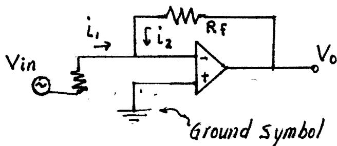
Output is measured from  $V_o$  to ground.
