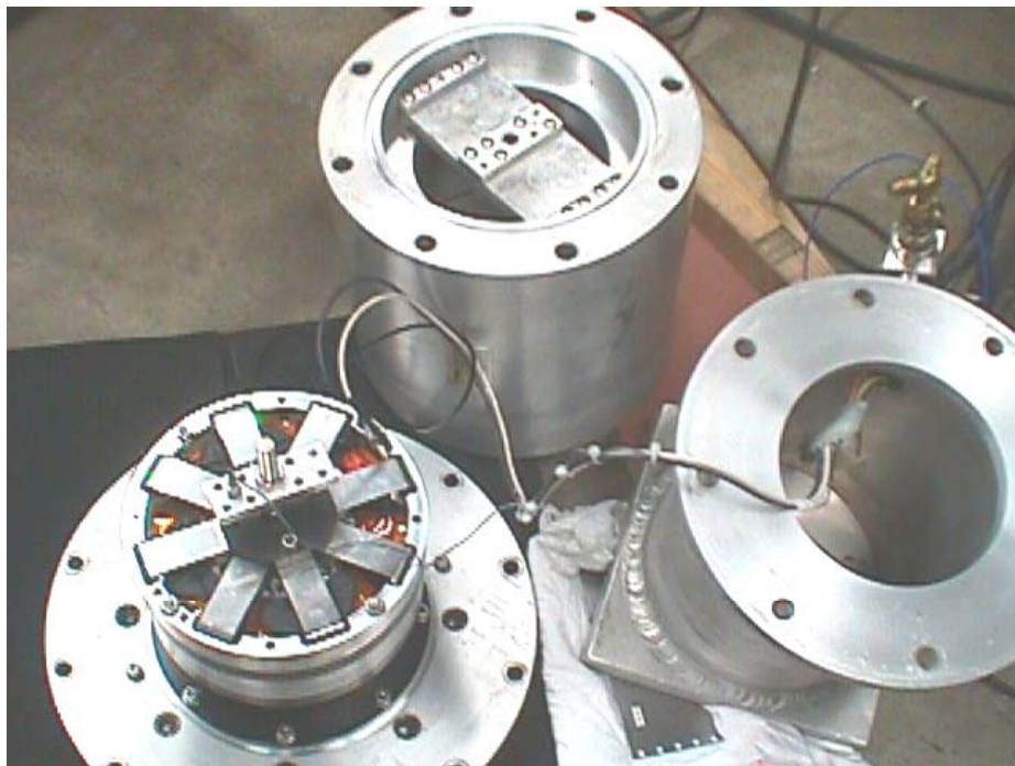
Figure 4: Picture of the Moving-Magnet Driver, Leaf Springs, and Enclosure.
