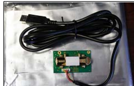
Figure 6: T6613/6615 CO 2 Sensor Connected to USB Cable
