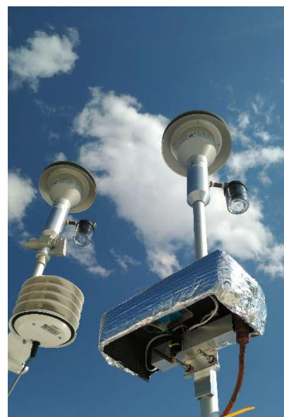
Figure 5: Experiment setup. Here, the instrument is attached to a BAM inlet pipe, where it was left to measure for the duration of the experiment.
