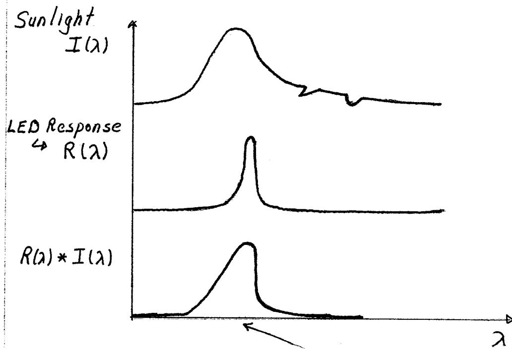
$V_{LED} = \text{Area under this curve}$
