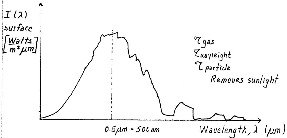
This is the spectrum of sunlight at the surface after it has passed through the atmosphere. Gas and aerosol particles absorb and scatter sunlight. Cloudy days have much more variable sunlight.
