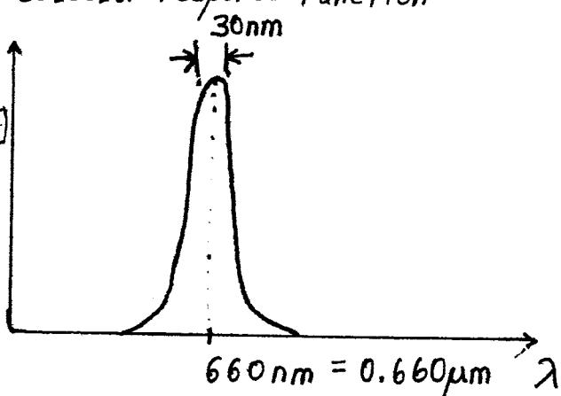
The Light Emitting Diode (LED) responds to light in a narrow wavelength band.
