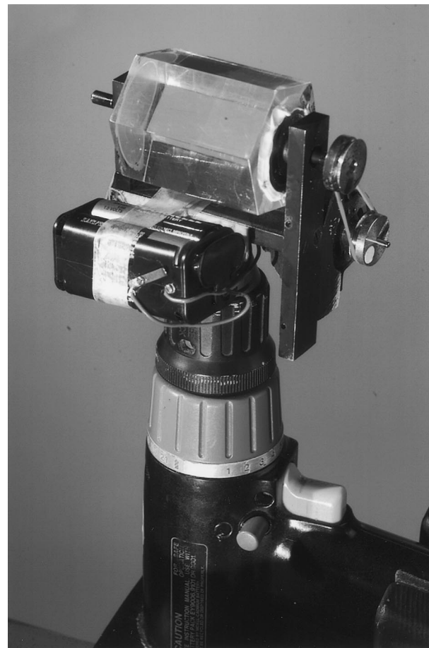
Fig. 5. Experimental arrangement for simultaneous rotation of hexagonal column crystals around two perpendicular axes.
